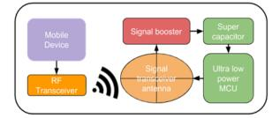
Figure 2: RF energy harvesting test bed
