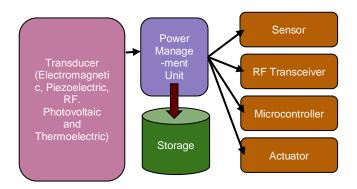
Figure 1: Block diagram of a typical energy harvesting system
